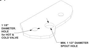
Should a counter top need to be drilled, please reference the diagram above.
