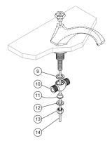
Install spout tee assembly (9, 10, 11, 12 and 13) as shown in diagram.
