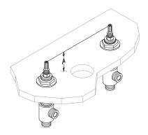
Set valve to proper rough-in height "A", by adjusting bottom-fastening nut. Secure valve by tightening top fastening nut \*YOU MAY NEED TO CUT THE ALL BROACHED STEM TO REDUCE THE VISIBILITY BETWEEN HANDLE AND ESCUTCHEON. Repeat procedure for the second lavatory valve. Please see page P99030A for the "A" measurement for your trim.
