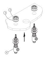
Remove top fastening nut and washer (2 & 3) from the lavatory valve. (NOTE A: All lever handle sets are supplied with one right-hand valve and one left-hand valve. Install valve with the blue dot on the cold side [Round handle sets are supplied with two hot valves that turn in the same direction]). Insert valve from below through hole in lavatory or countertop.
