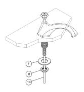
Insert spout base nipple into center hole in lavatory or counter top. Install stainless washer (7) and spont (8) on spout nipple and tighten. Place pop-up knob rod (14) though spout.
